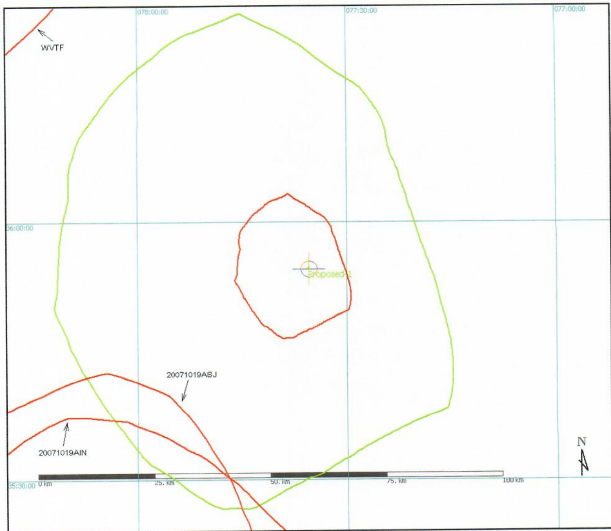
Illustration 15a(1): This map is color coded so that prohibited overlap is indicated by LIKE color contours overlapping.
